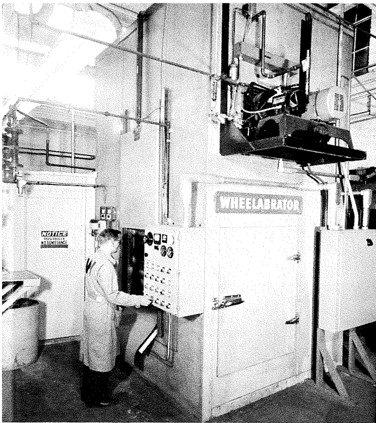
Robert Hatch, R & D Application Engineer, operates the Rubber Deflashing machine equipped with the new Frigibrator unit. The new unit eliminates use of costly carbon dioxide and liquid nitrogen in the deflashing process.
